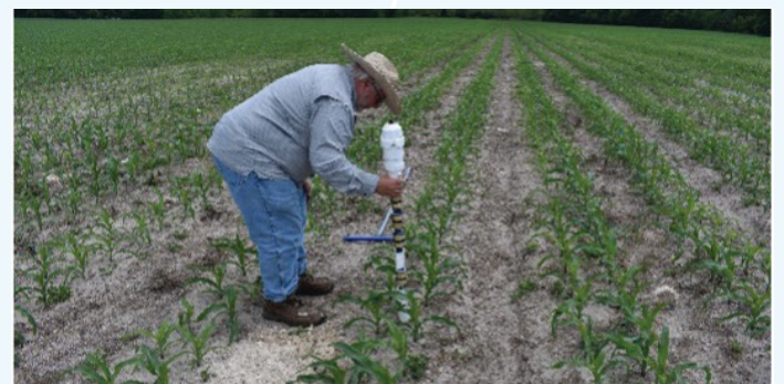
Figure 2. Joel Love, BMP outreach specialist, installs a soil moisture sensor for a corn grower. Photo by C. Barrett
