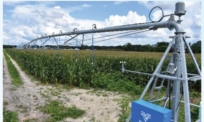
Figure 1. Center pivot irrigation system with low pressure drop nozzles increase crop water uptake efficiency. Photo by C. Barrett
