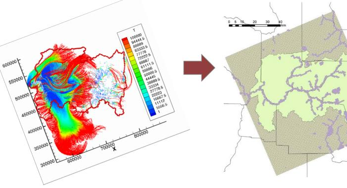
Figure 10: Particle tracking to establish groundwater flow boundaries into the Santa Fe River basin
