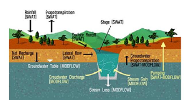
Figure 4: SWAT-MODFLOW hydrological tasks. Image courtesy of www.floridanwater.org
